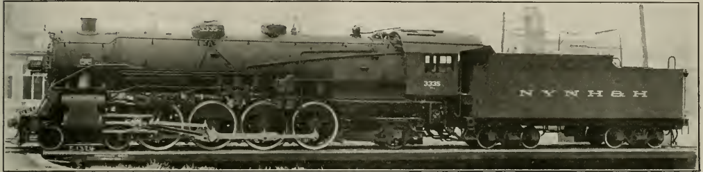
4-8-2 TYPE LOCOMOTIVE FOR THE NEW YORK, NEW HAVEN & HARTFORD RAILROAD AMERICAN LOCOMOTIVE COMPANY, BUILDERS
